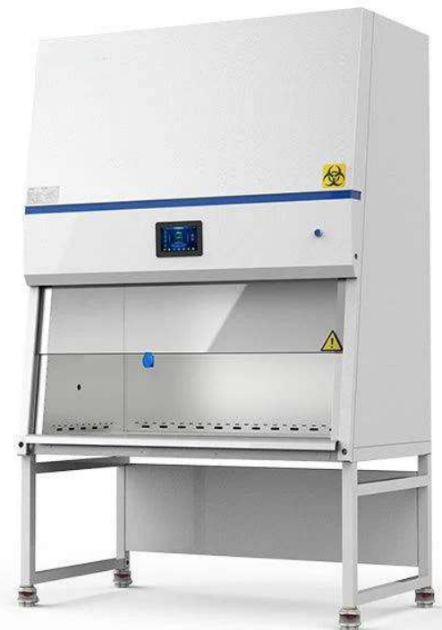
Class II, Type A2 Air in-flow 70% Recirculated vs. 30% Exhausted
