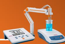
1-5 points calibration with Standard Recognition. Selectable pH buffer groups, including NIST, DIN, GB, USA. Automatic electrode diagnosis with pH slope and offset display.
