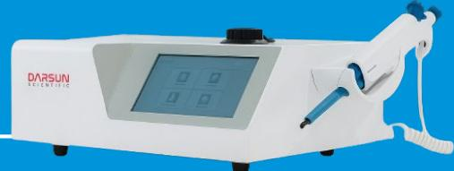
The blood coagulation analyzer adopts the principle of optical colorimetry for detection. After the reagent is mixed with the plasma, fibrinogen is converted into fibrin and coagulated, which leads to the change of the optical density of the test specimen, and the instrument detects the coagulation end point.
