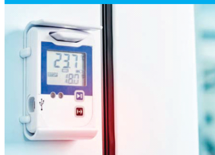
The data logger can be fixed to deep-freezers magnetically and configured or read via a USB interface
