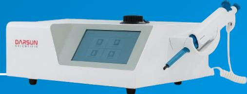
The blood coagulation analyzer adopts the principle of optical colorimetry for detection. After the reagent is mixed with the plasma, fibrinogen is converted into fibrin and coagulated, which leads to the change of the optical density of the test specimen, and the instrument detects the coagulation end point.
